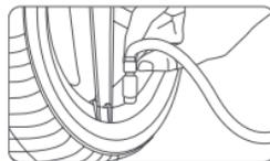
2. Turn on the device and place the on/off switch to “—” position to start pumping. If the pressure of the gas valve increases rapidly within a short interval (50 psi in 3 seconds), it means that the air way is obstructed. Please immediately turn off the power, detach the screw-on gas connector from the tyre nozzle and reconnect the gas tube.
