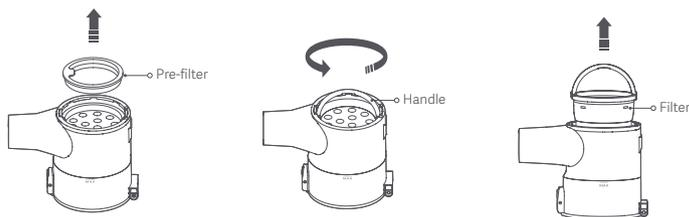
3. Rotate counterclockwise to remove the post-filter.
